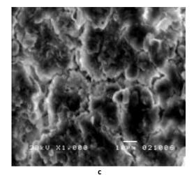
Figure 1: Scanning Electron Microscop of peat soil sample. a. peat soil without fly ash, with magnification 350 x, b. peat with 0.2 grams fly ash/10grams peat after two week incubation (500 x magnification) and c. peat with 0.2 grams fly ash/10grams peat after eight week incubation (1.000 X magnification).
