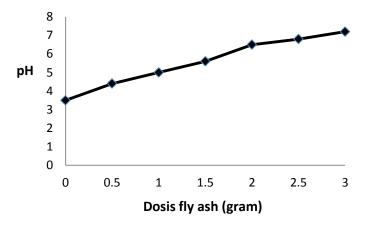
Figure 2: The effects of fly ash addition to pH of 10 g peat soil
